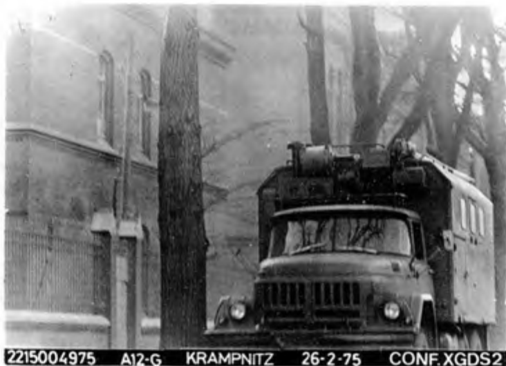
FTP-200 CBR FILTRATION SYSTEM ON ZIL-131
