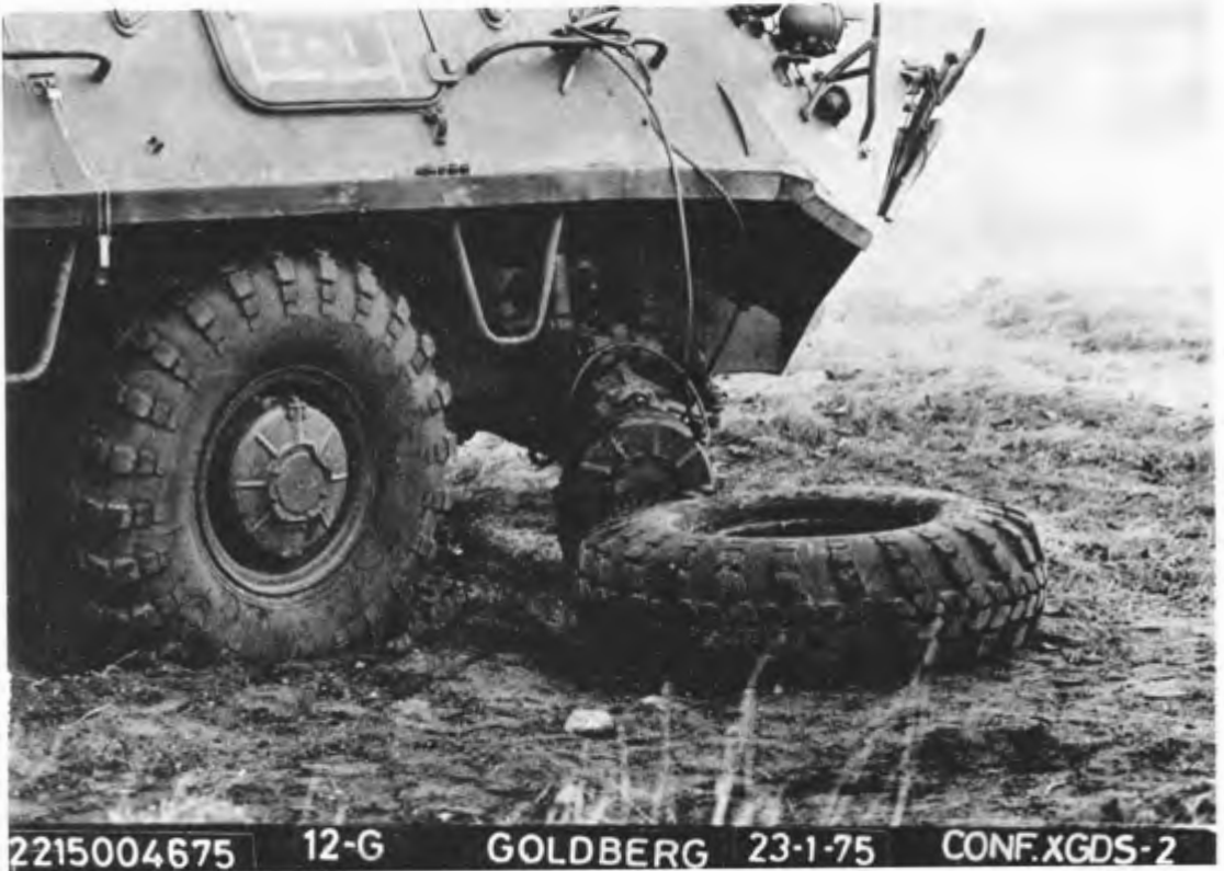
BTR-60PB EMERGENCY MAINTENANCE
